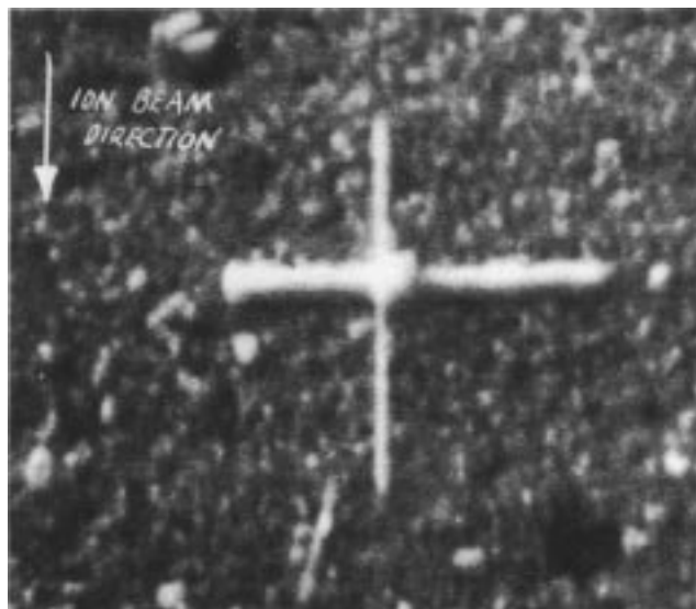
Figure 1. Scanning electron micrograph of a copper pattern formed by electron-beam lithography followed by image transfer using ion-beam etching. This structure, fabricated in 1964, was an early demonstration of the capabilities of nanolithography (Reprinted with permission from ref 5. Copyright 1964 Wiley and Sons.)
